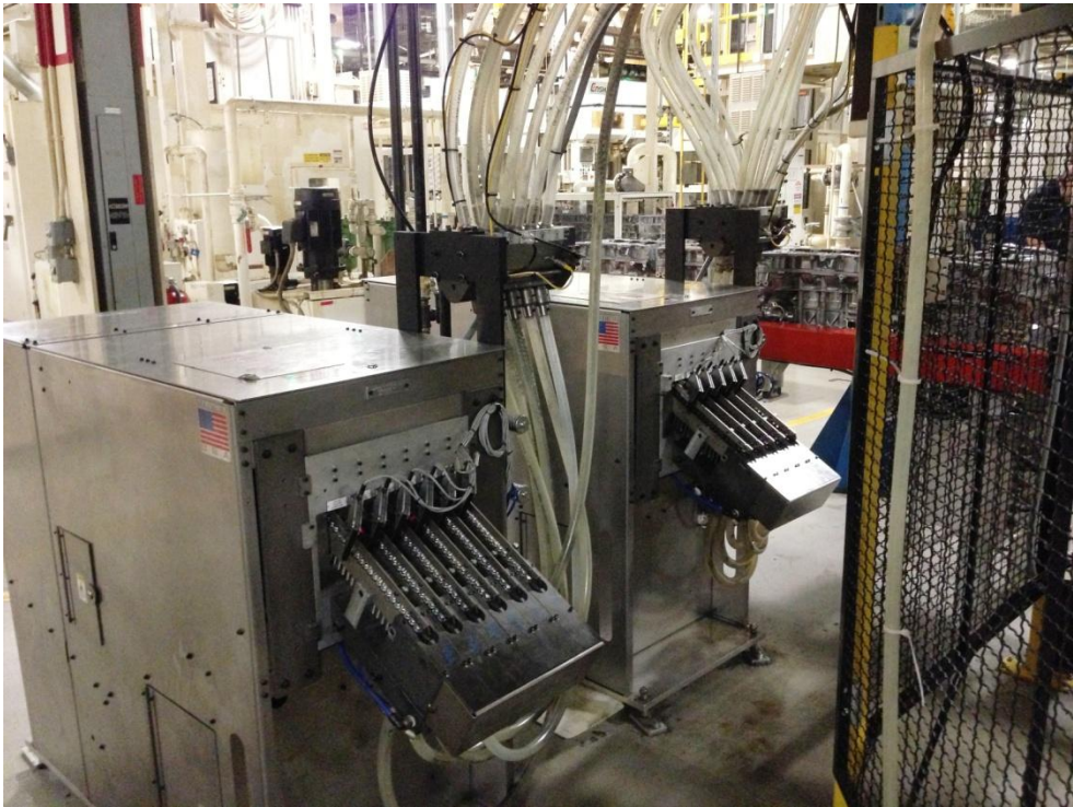
6 IN 12 OUT AND A 5 IN 10 OUT SET OF DIVERTERS MOUNTED TO OUR FEEDERS
