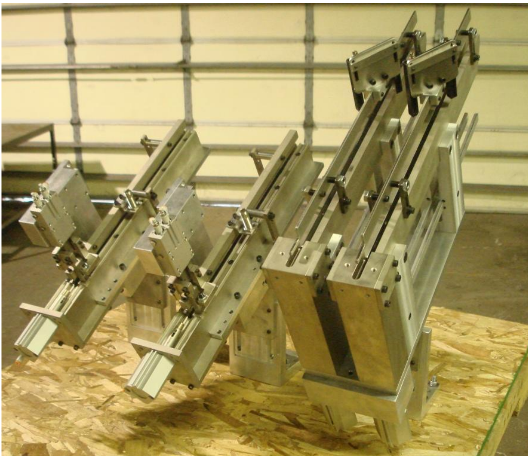
Manual load escapements for presenting detent pins and plates for robotic retrieval.
