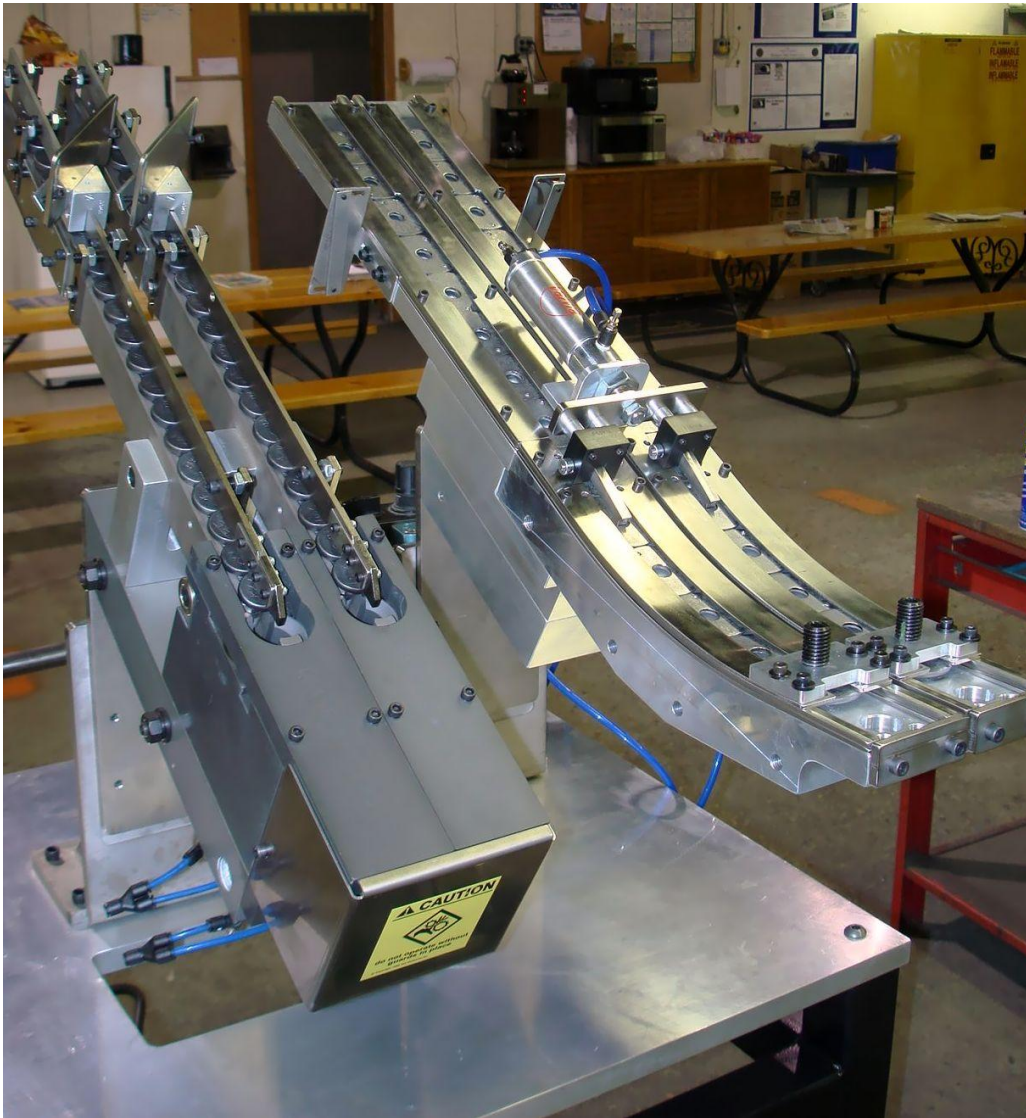
Manual load tracks and escapements for blow feeding weld studs and robotic retrieval of washers
