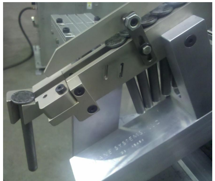
Presenting escapement for a headed pin. A robot comes in horizontally removes the pin from the spring loaded gate
