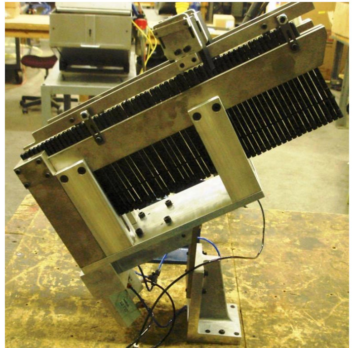
Presenting escapement for detent pins for shifter assembly
